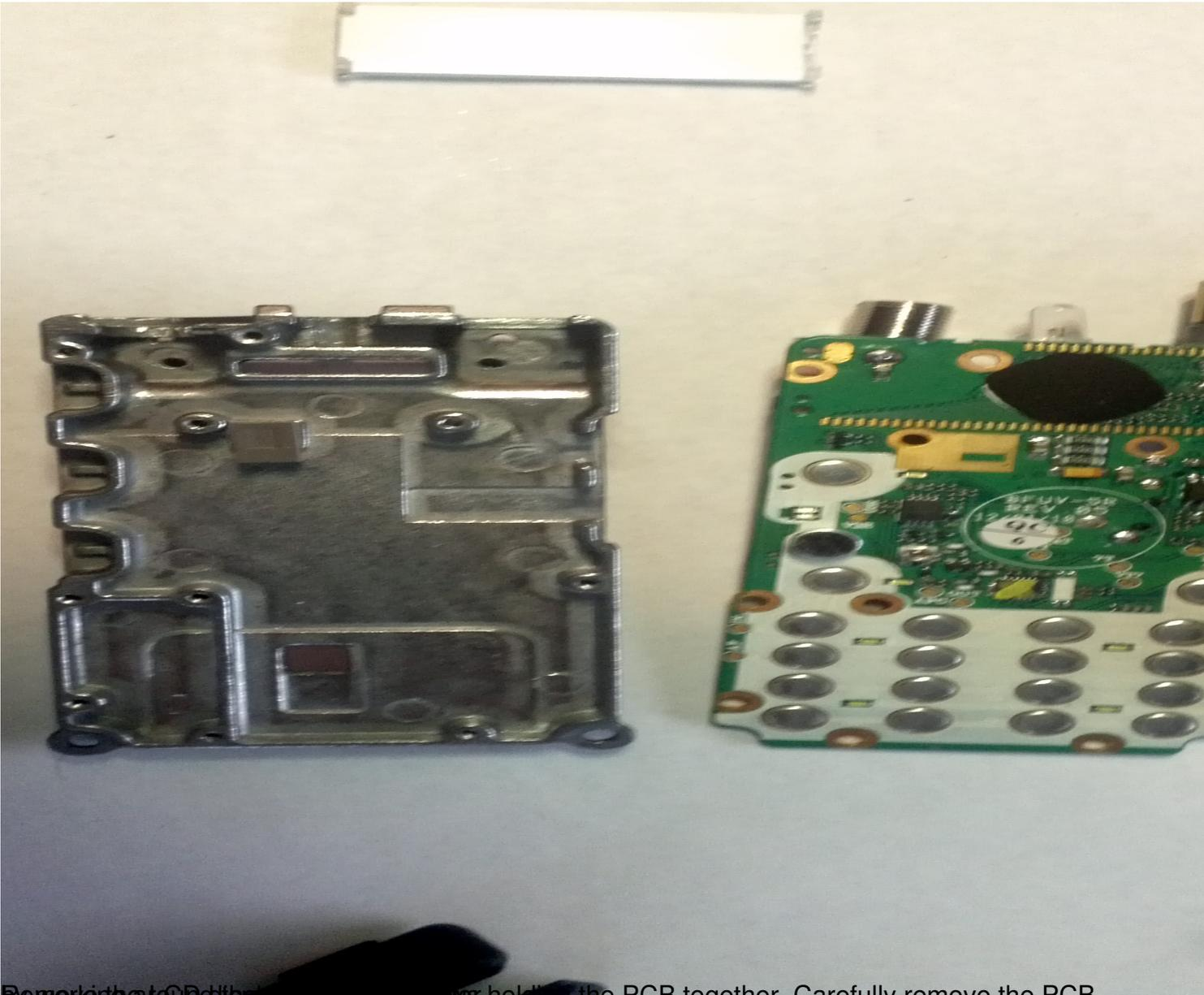
By moving the LCD display, and the screws holding the PCB together. Carefully remove the PCB
