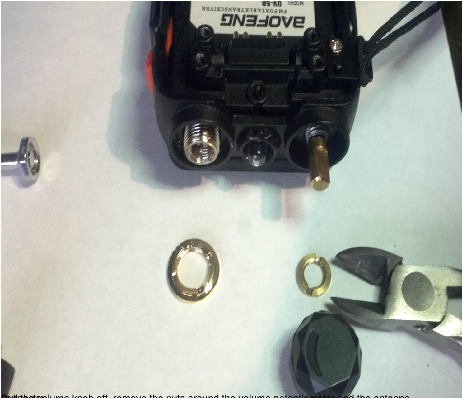
With the volume knob off, remove the nuts around the volume potentiometer and the antenna
