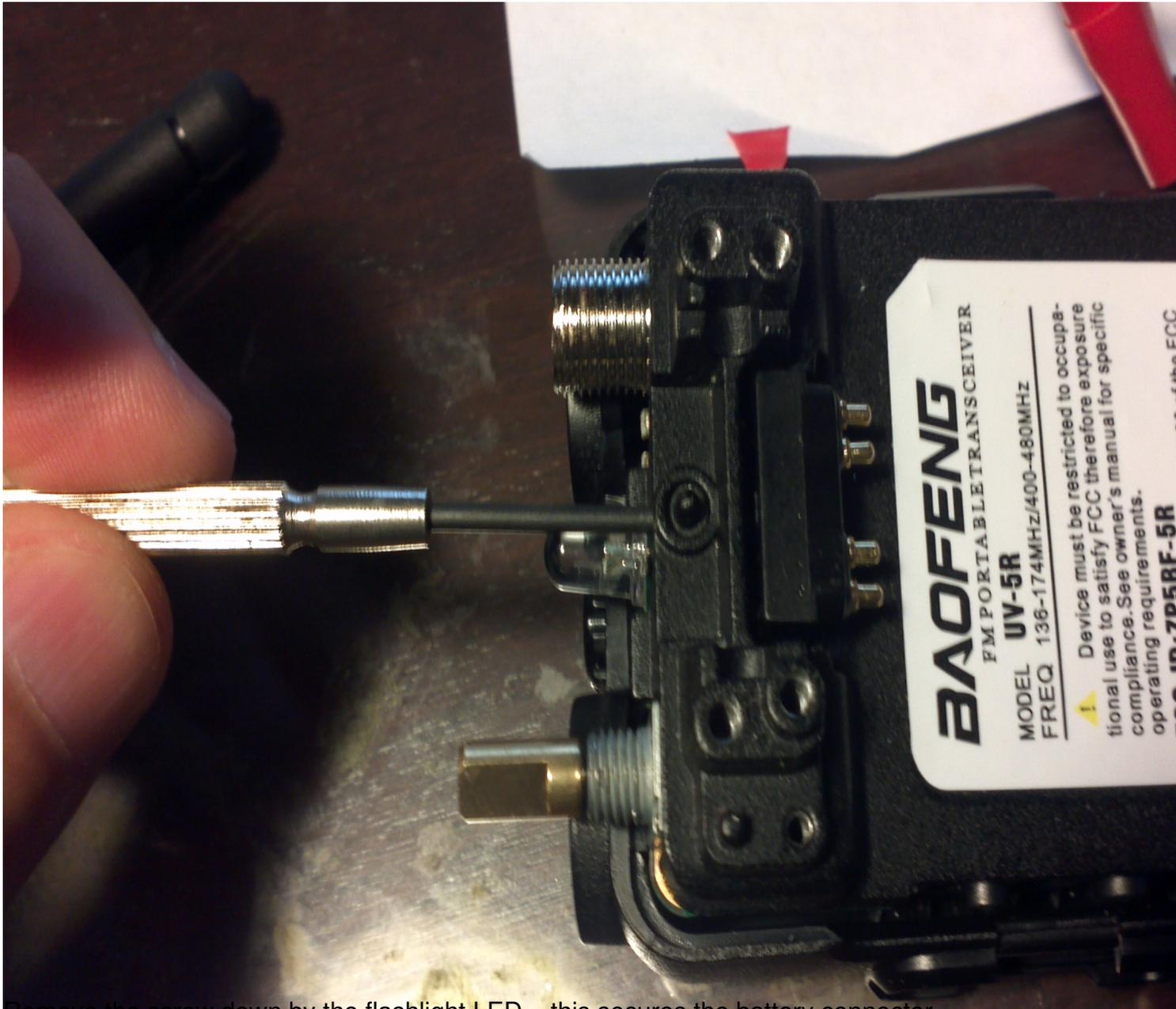
Remove the screw down by the flashlight LED – this secures the battery connector.
